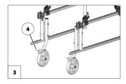
When parking the wheelchair the brakes of the shunting castors (4) are to be engaged.
