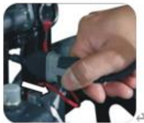
5. Remove the cable from the transmission connector.
