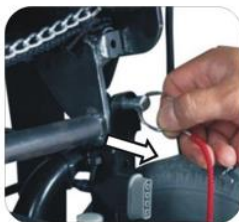
4. Pull the pins out from both sides of the mounting bases.↵
