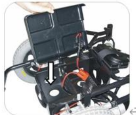
10. After removing the batteries, close the battery box cover.
