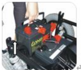
11. Lift up the battery by its handle.
