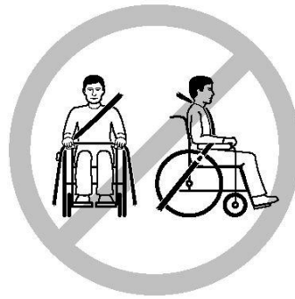
Incorrect seat belt position
